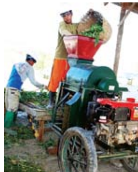
Organic waste being turned into compost
