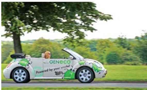
The Bio-Bug, developed by Wessex Water subsidiary GENeco, runs on biogas generated from the sewage treatment process
